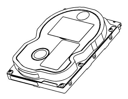
Horizontal mounting with the PCB facing down
